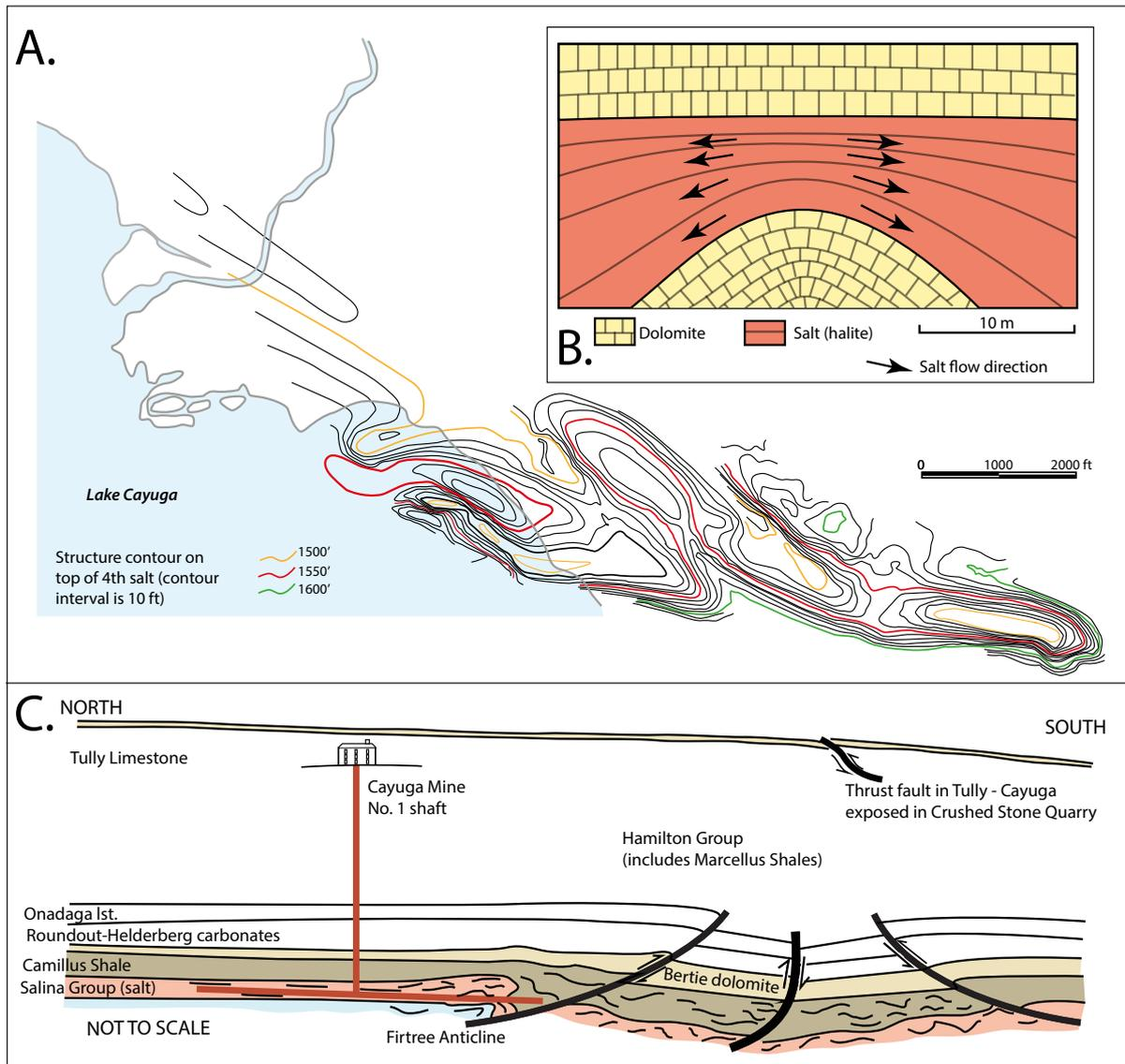
Figure 11. Salt geology in the vicinity of the Cargill-Cayuga mine. A) Structure contour (in feet) on top of the “4th” salt, this is top D in the current terminology. B) Illustration of the ability of salt to flow, while adjacent interbeds do not, so illustrating one mechanism for lateral changes in salt thickness. C) Interpretive schematic based on regional thickness changes seen in wells and observations in the Cayuga Mine (after Prucha, 1969; Goodman and Plumeau, 2004a, b)
