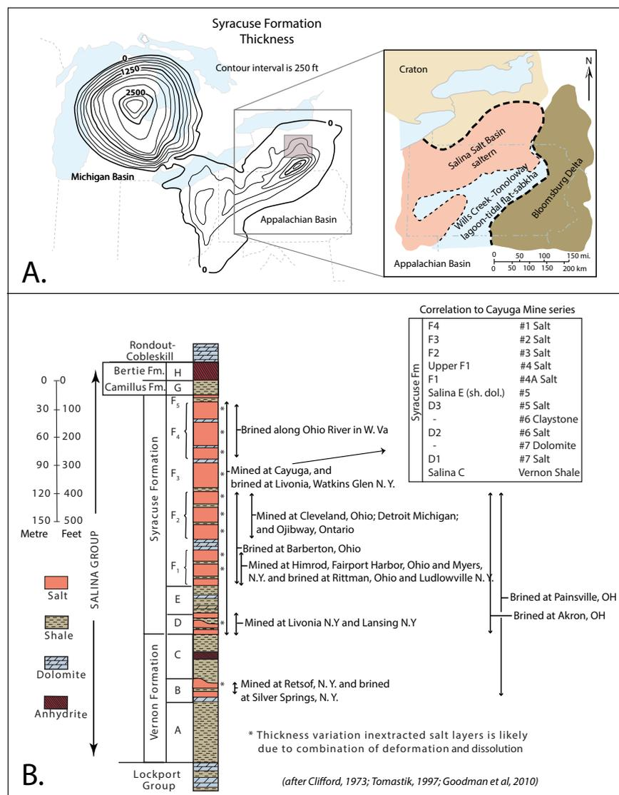
Figure 1. Extent and stratigraphy of salt in the Silurian Salina Group in the northeast USA. A) Distribution and thickness of salt in the Salina Group. B.) Figure 5. Stratigraphy (rock unit names) used to describe salt units in New York State and surrounds, along with a listing of targeted salt intervals in former and current mining or brine well operations across the region. Insert gives the correlation of the regional stratigraphy to units used in the Cayuga Mine.
