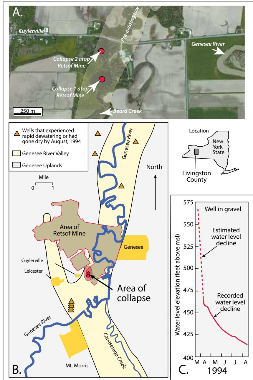
Figure 4. Retsof Mine collapse (after Warren 2016b). A) Location of the collapse dolines atop the former Retsof Mine to the east of the town of Cuylerville. The doline occupies a pre-existing low that had also captured Beard Creek (Bing® 2012 image mounted and scaled in MapInfo). B) Locality and areas of collapse with effects on the landscape, along with a hydrograph from a well showing lowered water table in the Genesee River Valley (March 12 to August 12, 1994; after Tepper et al., 1997).
