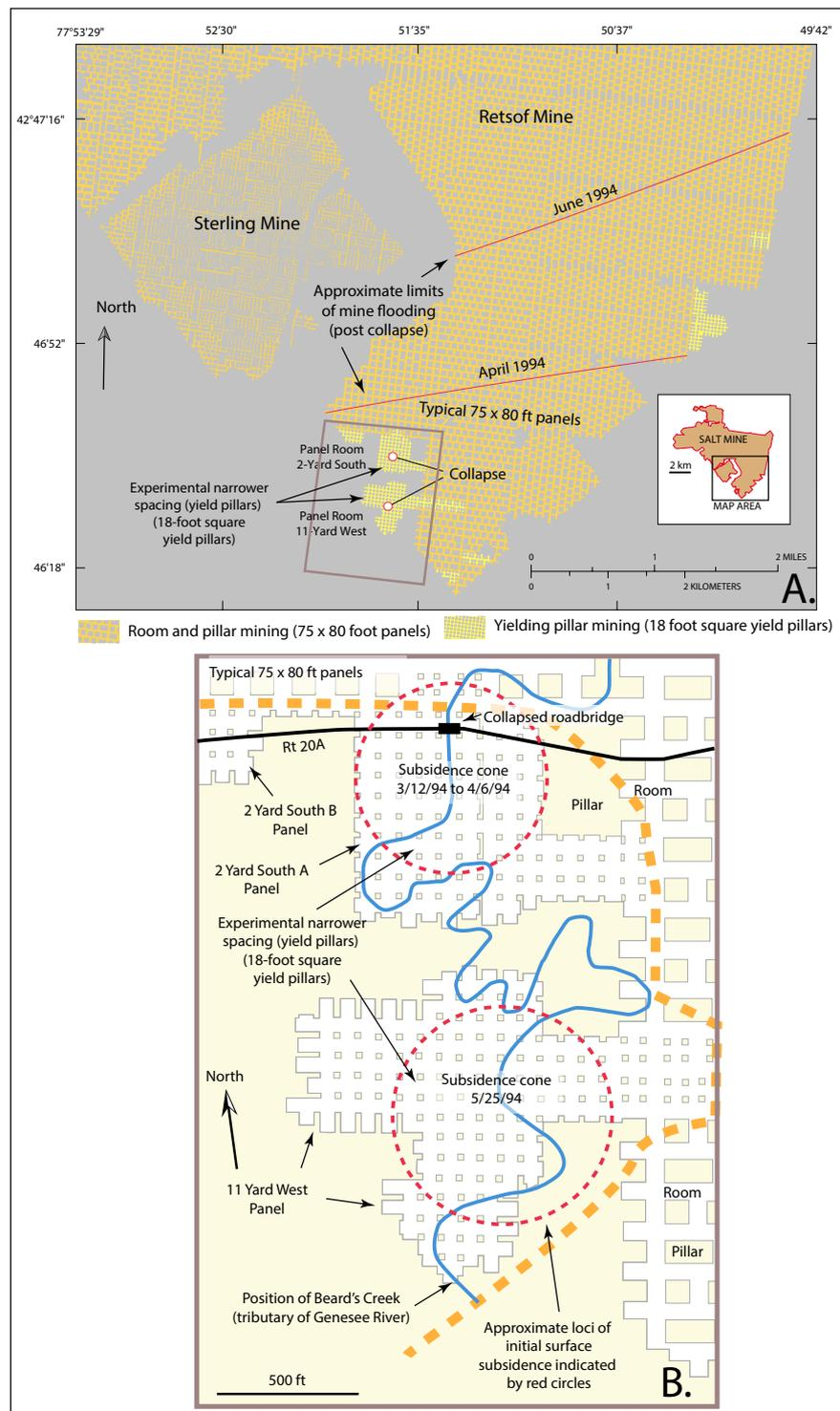
Figure 3. Retsof Mine. A) Room and pillar structure in the southern extent of the Retsof Mine at the time of the roof collapse and flood, also shows the position of the water flood edge after the collapse (after Yager et al., 2001). B) Detail of the new yield panel area and design at the time of collapse and its position relative to subsequent collapse features at the landsurface (after Nieto and Young, 1998; see also Figure 4).
