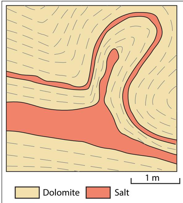
Figure 12. Field sketch of the geology visible in a mine wall showing clearly that the distribution of non-salt beds in the rocksalt is clearly not horizontal (after Prucha, 1968)
