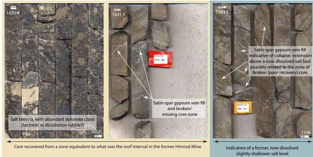
Figure 9. Rock-core based observations relevant to the nature of the top of a salt unit and indications of former, now dissolved salt levels in the Cayugan salt of the Salina Group. (Images downloaded from <[http://esogis.nysm.nysed.gov/Cores\\_TOC.cfm](http://esogis.nysm.nysed.gov/Cores_TOC.cfm)>, last accessed Dec.,2016).
