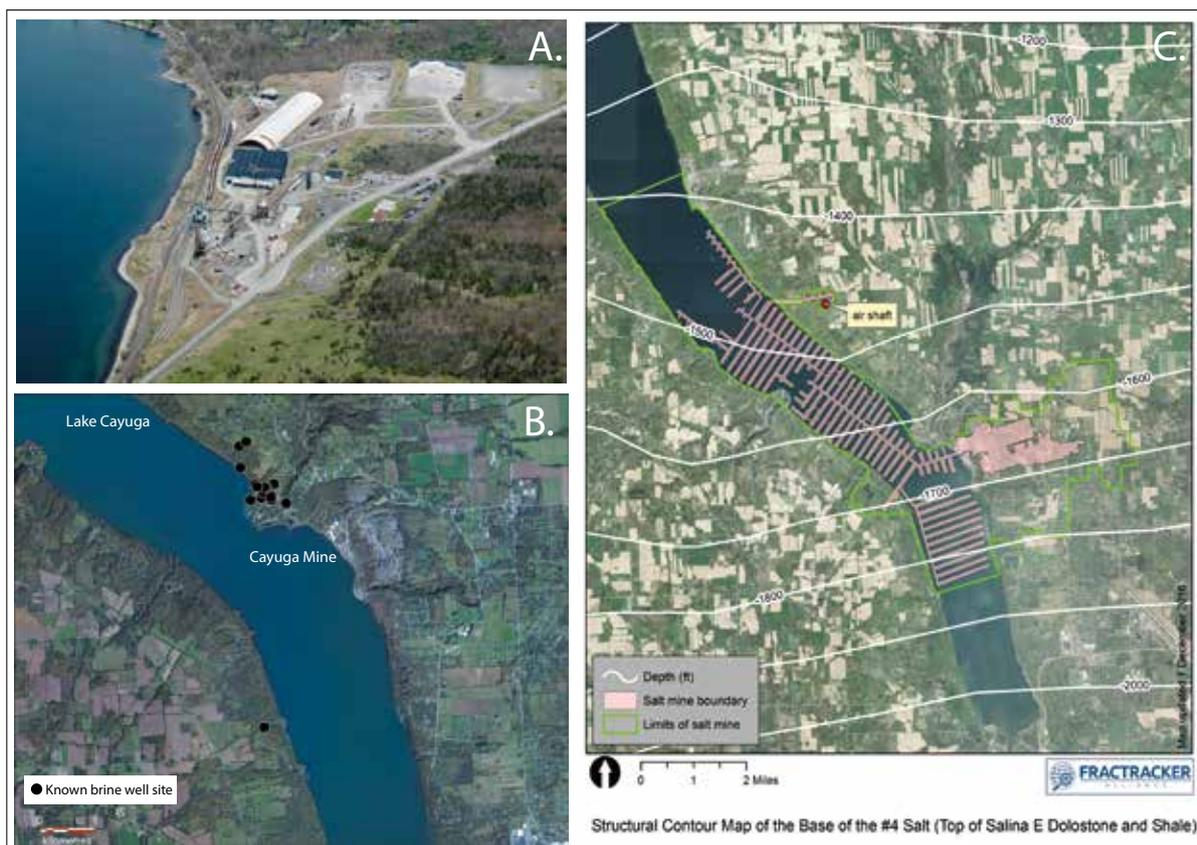
Figure 10. Cayuga Salt Mine, New York State. A) Current lake shore position of Cargill Salt's main shaft and surface operations. B) Positions of documented brine wells ranging in age from the 1890s until the 1970s and extending to depths of more than a kilometre. C) Approximate extent of current mine workings beneath Lake Cayuga and contour of base Salt #4; Image courtesy of FracTracker).
