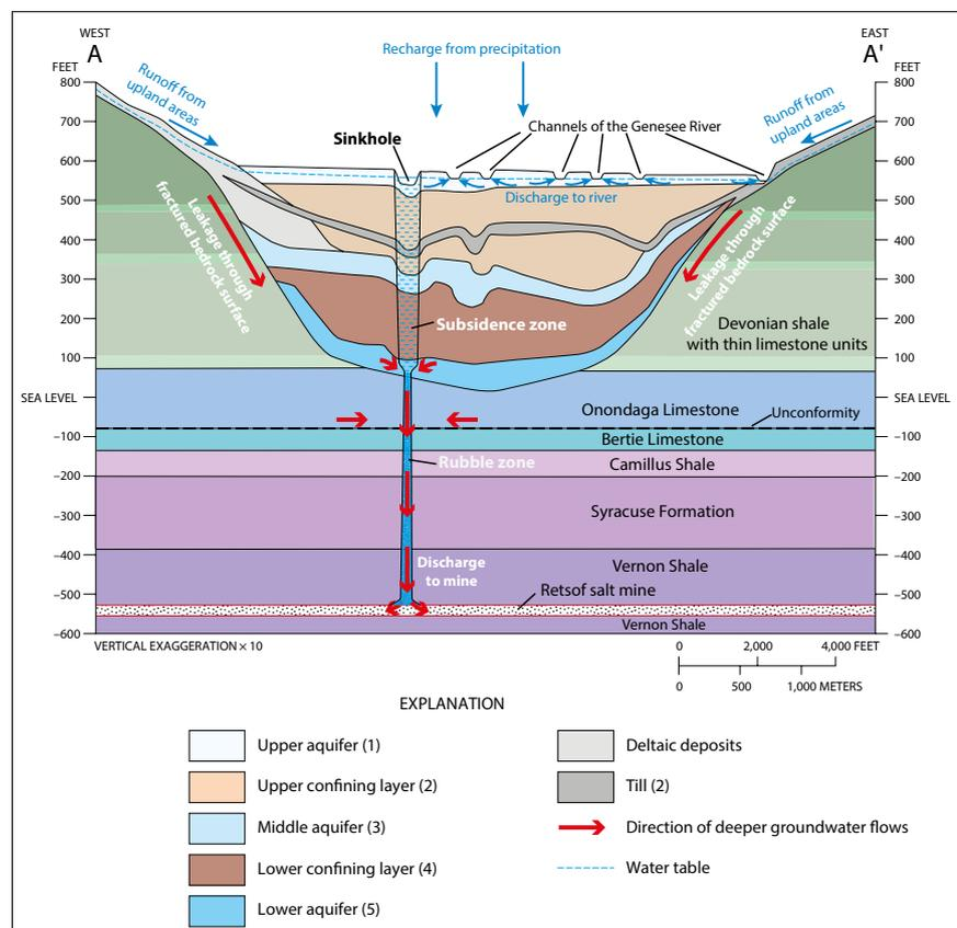
Figure 6. Stratigraphic section depicting rubble chimney above collapsed room in Retsof salt mine, Livingston County, N.Y. Also shown are the main aquifers that facilitated water influx into the flooding mine (inflow also drained natural and artificial brine-filled solution cavities in the stratigraphic levels above the working mine level (after Yager et al., 2009).
